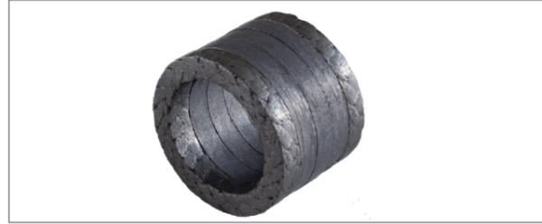
**Merkel Valtec 7888** packing set is based on engineered end rings braided by wire reinforced expanded pure graphite yarns. The middle rings are based on uniquely impregnated expanded graphite rings in different densities. All single components are additionally impregnated to further improve sealability and frictional behavior.
