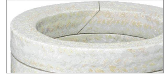
Merkel Arostat is made of wear-resistant and flexible aramid yarn. The packing is thoroughly impregnated with PTFE. This results in a very dense and resilient structure making Merkel Arostat particularly ideal for housing and cover lid applications.
