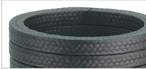
**Merkel Unival** consists of graphite-filled lubricated PTFE yarn. The special braiding structure offers the benefits of low thermal expansion and excellent heat conduction. Due to its low friction characteristics Merkel Unival can also withstand dry running up to a certain limit. In addition, its pliable and dense composition allows Merkel Unival to seal effectively with a minimum of gland pressure. The packing is approved for use in the food processing industries.
