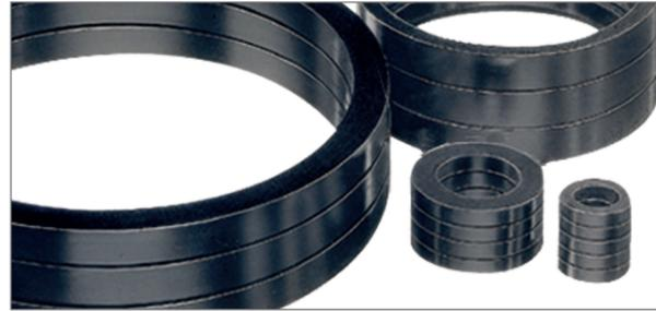
Merkel Grafiflex is characterized by a high level of chemical resistance and thermal stability as well as excellent sealing effect and constant elasticity. Regardless of temperature cycle this material is not subject to cold flow, shrinkage or aging. Merkel Grafiflex fulfills the purity requirements for seals in nuclear power station valves (content of soluble chlorides < 20 ppm).
