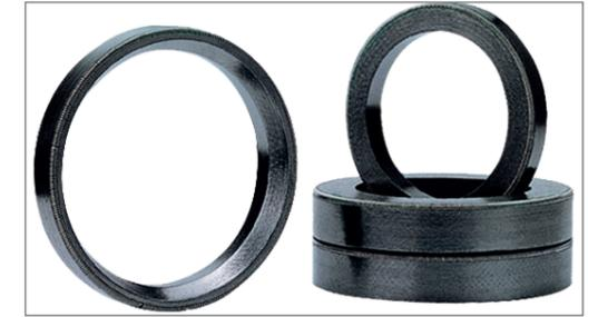
Merkel Grafiflex-cover seals are supplied as preformed rings and offer proven high performance, especially in heavy-duty valves or high-pressure feed-water pre-heaters. Merkel Grafiflex remains elastic even with fluctuating temperatures and pressures up to 200 N/mm<sup>2</sup>. Clearances up to 0.3 mm can be sealed without difficulty. Larger gaps can be controlled by Merkel Grafiflex reinforced with stainless steel springs or caps integrated into the corners.
