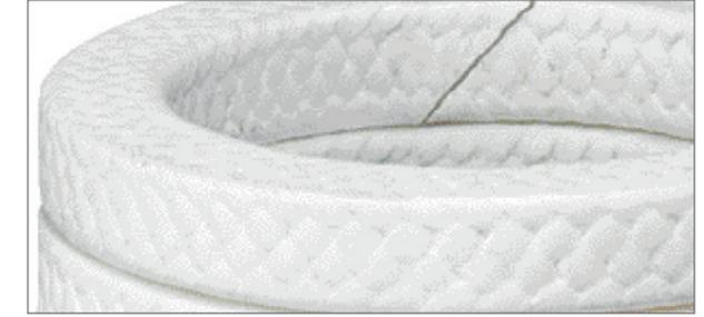
**Merkel Alchem** is manufactured from pure PTFE yarn with an additional PTFE impregnation, ensuring excellent chemical resistance. Its high density and tight braid structure ensure very low leakage performance. The packing has a high degree of form stability and a low compressibility which makes it also suitable for plunger pump applications. The packing is approved for use in the food processing industries.
