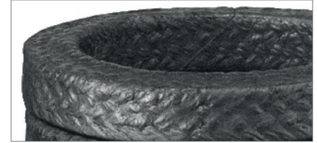
Merkel Uniflex is manufactured from a carbonized yarn with a special PTFE-graphite impregnation. The packing is very flexible and extrusion-resistant. The impregnation maintains an excellent bond to the yarn over the complete life of the packing. The thermal and volumetric stability provides superior sealing performance with minimal gland compression. These features make Merkel Uniflex suitable for use in "dry-running" applications.
